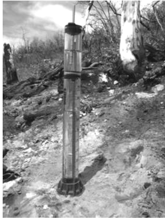
Fig. 2.8. The Mini-Disc Infiltrometer by Decagon Devices. Pullman, WA.
