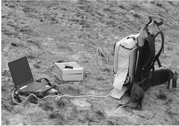
Fig. 2.9. The FieldSpec Pro by Analytical Spectral Devices.
