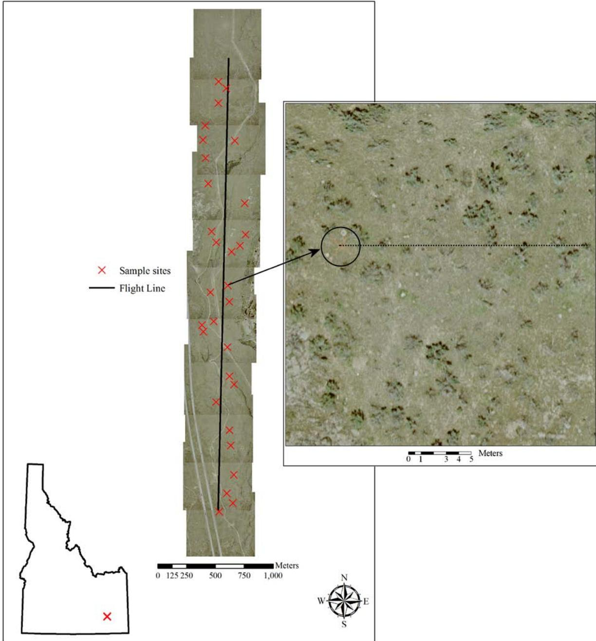
**Figure 1. The flight line and 50-mmpp VLSA imagery collected at the O'Neal Ecological Reserve in 2009. Inset shows an example of the imagery and illustrates the red-X painted on the ground (circled). The black dots extending west to east indicate the location where point observations and corresponding API observations were made.** *Aerial Photography Acquisition*
