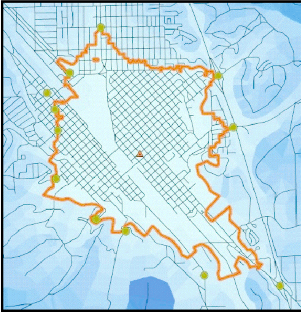
Figure 12. This figure shows how the calculated response time (line), for fire station 1 in Pocatello, compares to the tested response time (points).
