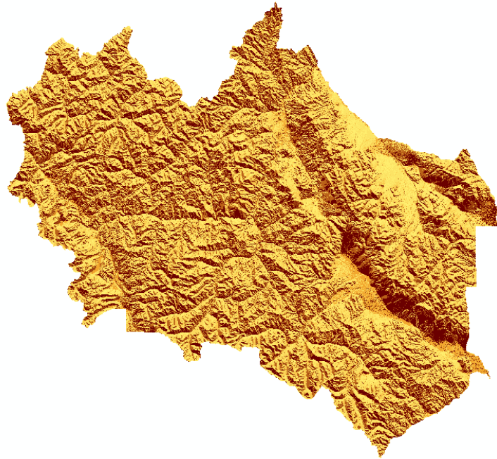
FIGURE 10 - THE SLOPE/SUPPRESSION DIFFICULTY COMPONENT MODEL. THIS MODEL EXPRESSES HOW DIFFERENT SLOPE STEEPNESS AFFECTS FIRE SUSCEPTIBILITY. DARKER COLORS INDICATE AREAS WITH HIGH VALUES FOR THIS MODEL.
