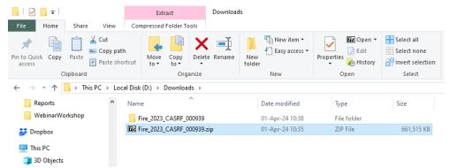
5. Navigate into the new folder to explore its contents. Since these files have been extracted to your computer they are ready for use by other software installed on your PC (e.g., ArcGIS Pro).
