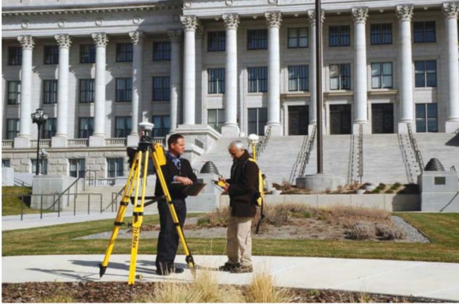
Sean Fernandez (left) and Hussein Yazdani collect position data at the Utah State Capitol. The GNSS receiver on the tripod is measuring a geodetic control monument used to monitor the accuracy of TURN GPS. Photo courtesy Utah AGRC.
