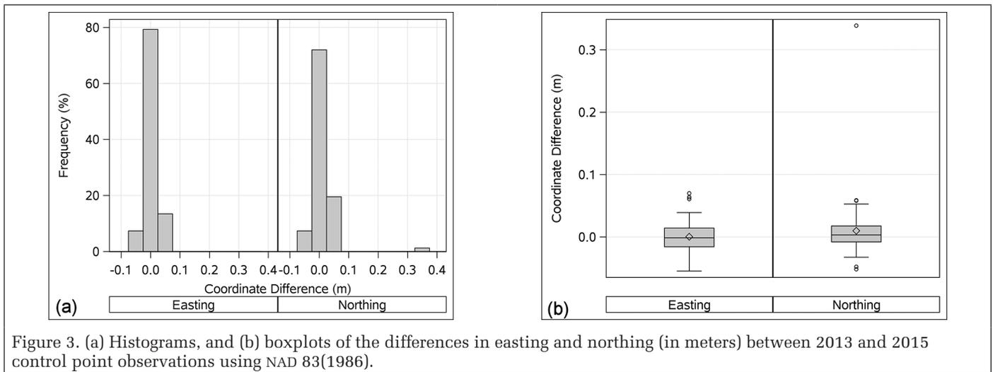
Figure 3. (a) Histograms, and (b) boxplots of the differences in easting and northing (in meters) between 2013 and 2015 control point observations using NAD 83(1986).
