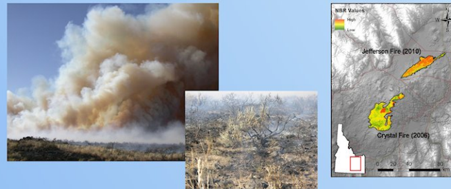
Figure 4. The Normalized Burn Ratio (NBR) for the Crystal and Jefferson Fires. NBR was calculated with atmospherically corrected Landsat 5 TM imagery using:
